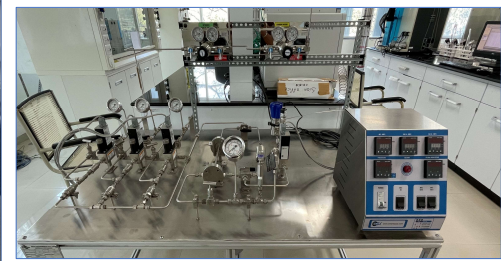
High pressure, high temperature, multi-phase flow-storage-deformation studies including the dynamic breakthrough
